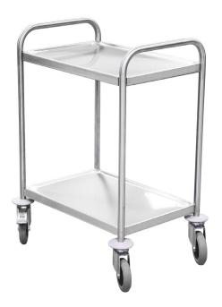
Rugged construction made from two tubular steel bar push handles,  $\emptyset$  25 mm, with welded deep drawn shelves with elevated perimeter flange in-between. Deposit surface with large radii for easy cleaning, lowered by approx. 10 mm in contrary to the perimeter flange. Shelves are bevelled by 35 mm all over, with flat safety return to the inside and sound absorbing lining.
